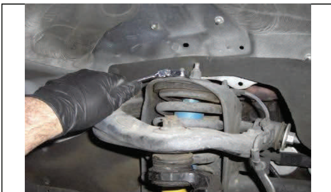
Disconnect upper strut mounting hardware
