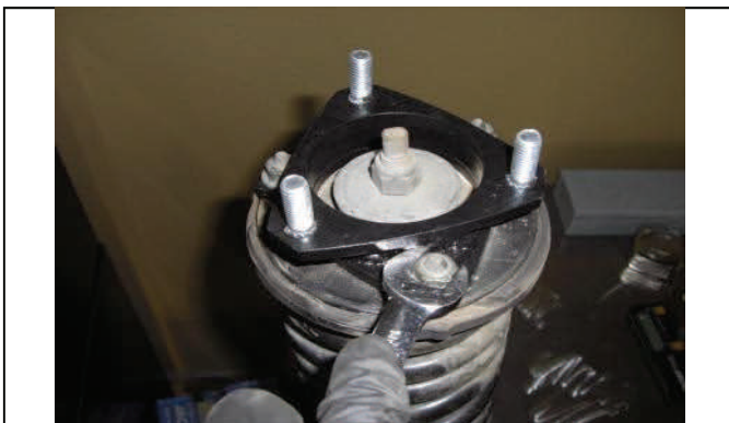
Attach new strut extension with OE hardware
