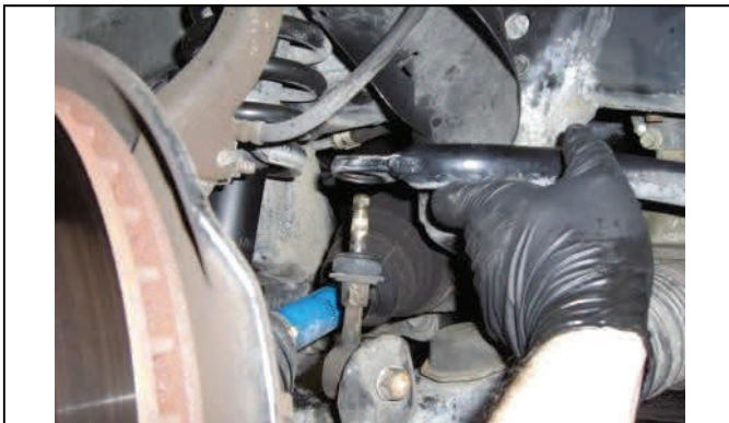
Shows earlier model sway bar end links
