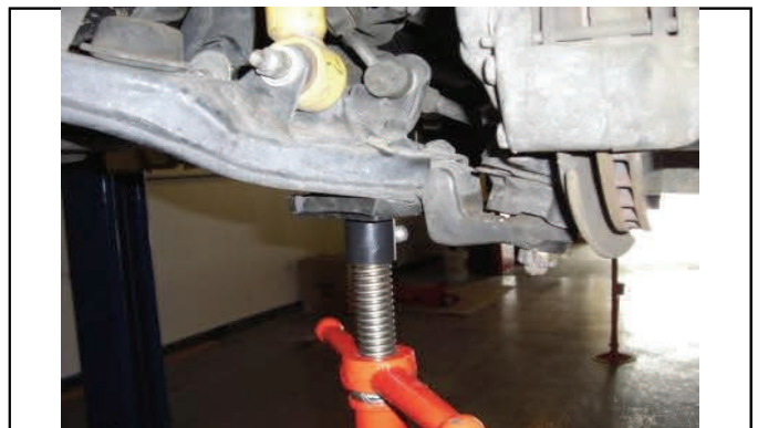
Raise lower control arm and attach lower strut mount
