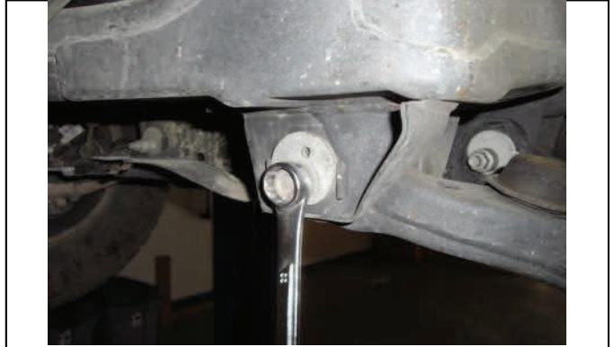
Reset and tighten lower control arm bolts
