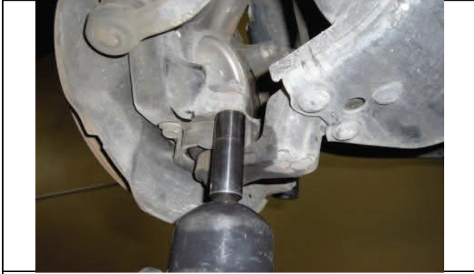
Reattach lower ball joint bolts and tighten
