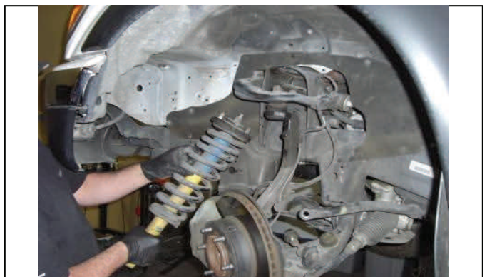
Remove strut from vehicle
