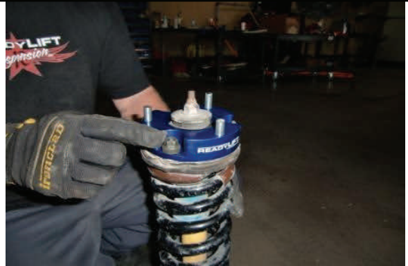
Attach assembled spacer to top of strut w/ OE hardware
