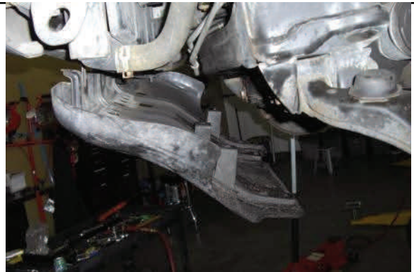
4WD models remove front skid plate
