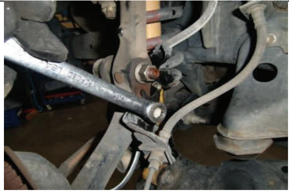
Disconnect ABS/brake line bracket at spindle
