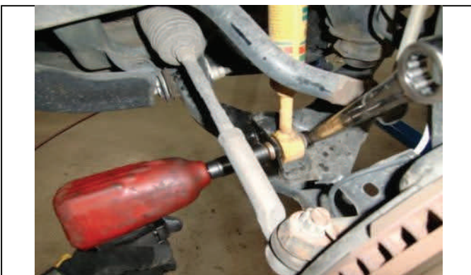
Remove lower strut mounting hardware
