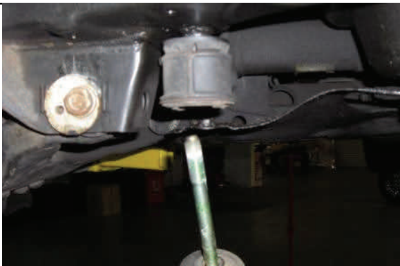
4WD Support differential & remove front mounting hardware
