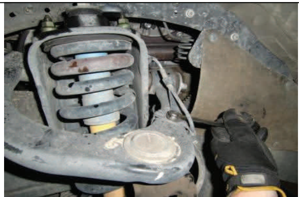
Disconnect ABS/brake line upper bracket
