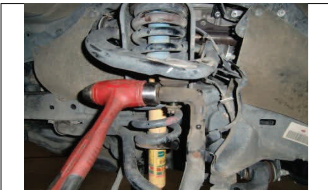
Loosen upper ball joint nut and strike to disconnect
