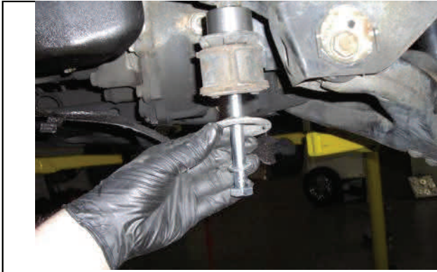
4WD Install longer bolts and reattach differential to frame
