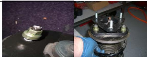
5. Rotate the top of the strut 120 degrees so that when you install it the bracket on the bottom of the strut is on the is back in the stock location.
