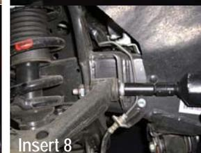
3. Loosen, **DO NOT REMOVE**, the lower control arm nuts. Be sure to mark the alignment cams and the flanges they contact. (Insert 9)
