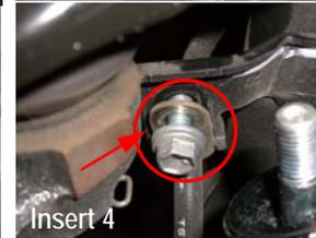
2. Remove the upper 12mm sway bar end link nut and 17mm lower end link nut. Remove the end link. (Insert 5 & 6)
