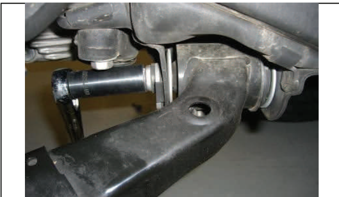
Loosen both lower control arm pivot/alignment bolts
