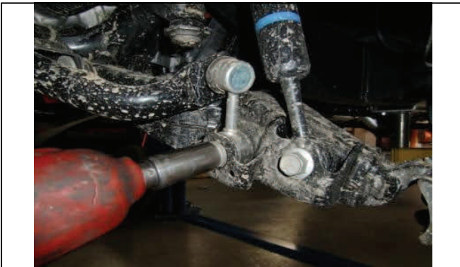
Disconnect lower sway bar end links
