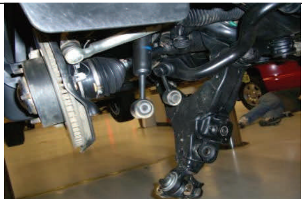
Swing down lower control arm and remove strut
