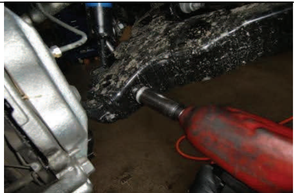
Remove lower strut mounting hardware
