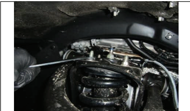
Remove upper strut mounting hardware
