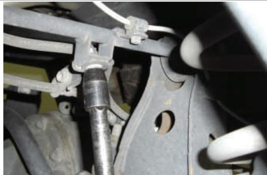
Remove the rear wheels. Unbolt the brake line support bracket bolt located on the driver side rear upper trailing arm.
