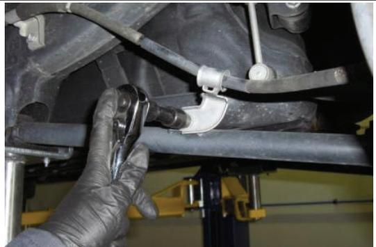
Remove the emergency brake line support bracket bolts located on both the driver and passenger side lower trailing arms and on the frame rail.
