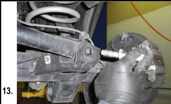
Unbolt the lower panhard bar. Remove the rear coils and bump stops.
