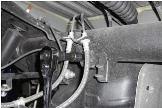
Remove the brake line support bracket bolt located on the cross member near the fuel tank.
