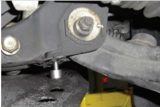
Re-install the skid plate using the OEM hardware in the front and the supplied hardware in the back. The 1/2" tall spacer goes between the frame and the skid plate.
