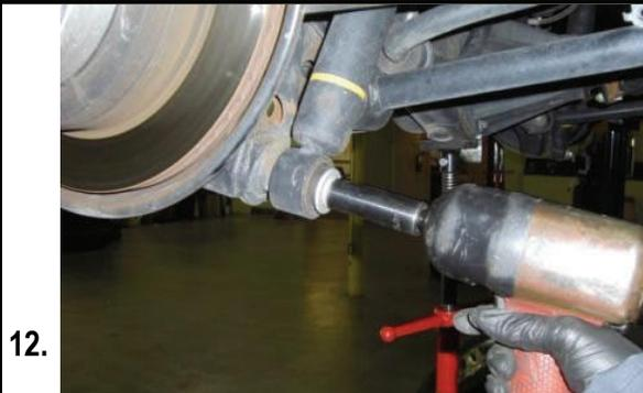
Unbolt the lower rear shocks. Unclip the ABS line at the various points that need slack as you lower the axle.
