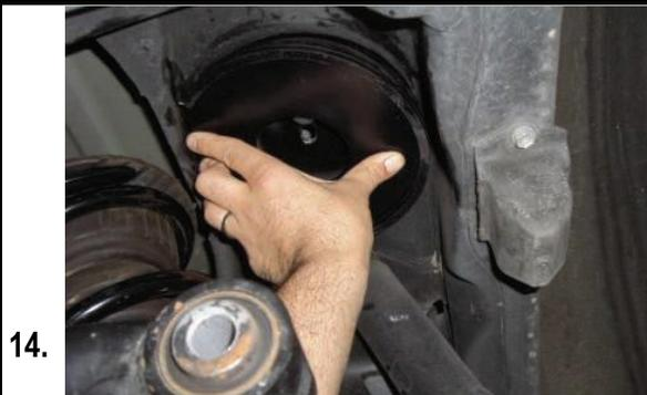
Install the ReadyLift rear coil spacers using the M14 hardware supplied. Torque to 95 ft-lb.
