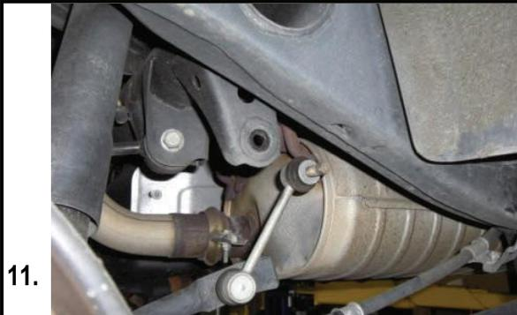
Unbolt the upper sway bar end links. Support the rear axle with a jack.
