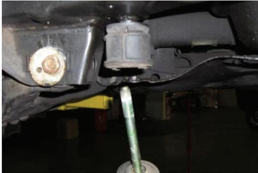
Remove the front skid plate and save the OEM hardware. Support the front differential with a jack and remove the two differential torque arm bolts. Save the large washer.
