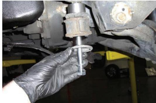
Slowly lower the jack to allow the differential to rotate down. Place the 1" tall steel spacers between the frame and torque arms. Install the supplied hardware with the large washer.
