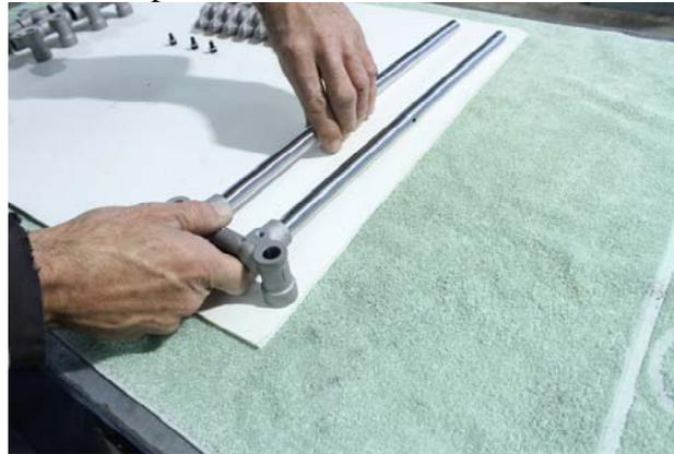
5. Loc-tite the allen bolts and using the zinc washers, screw them in to secure the shaft inside the stand
