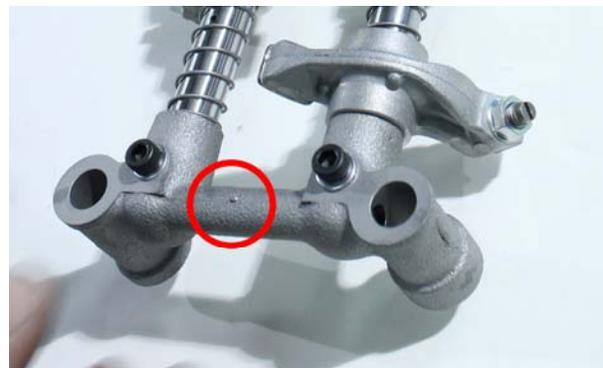
3. Install the valve adjust screw, with the flat side towards the valve tip. After that, install the nut on the upper part of the valve adjust screw.
