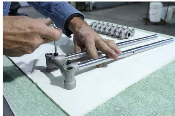
6. Following the pattern of the valves on the cylinder head install the first two springs and two rockers arms. (Alternating between spring and rocker arm) **(This will be for cylinder #4).**
